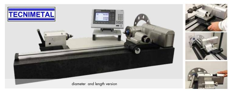
GIOTTO-MAN is a manual measuring bench for shafts designed to be placed in the production floor for an immediate feedback on the tolerance limits. Diameter and Length measurement axis are activated by operator. The repeatability is ensured by a dedicated mechanical system.
